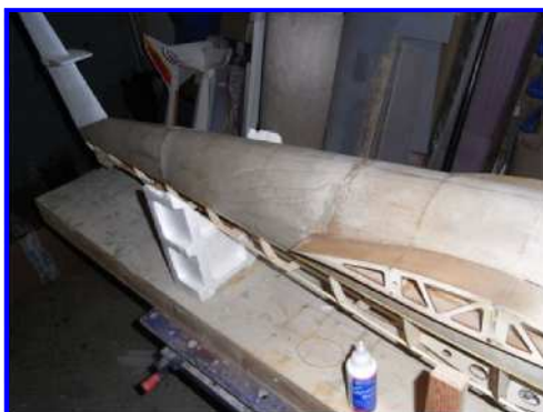
Top back covered. None of the forward planking was done yet.
