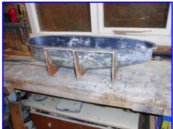
Female mould ready for the plaster.
