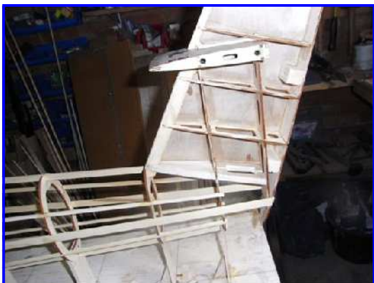
Fin fit. You can see the extra thick rib. This is a trial fit. I removed the fin and added the sheeting before gluing it in.
