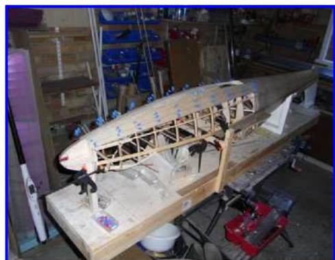
Back covered, planking up, front going in. Nose formers and tow release are visible.
