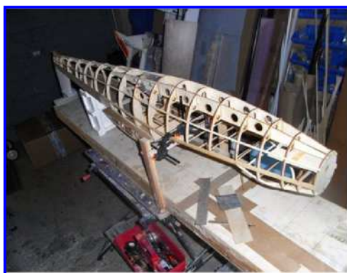
Fuselage inverted ready for planking
