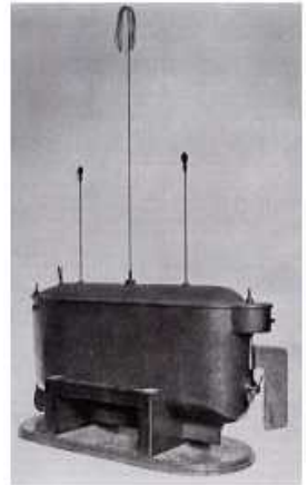
In 1898, Tesla demonstrated a radio-controlled boat (U.S. Patent 613,809 — Method of an Apparatus for Controlling Mechanism of Moving Vehicle or Vehicles).
