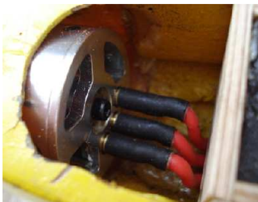
Electric Cables connecting at rear of motor
