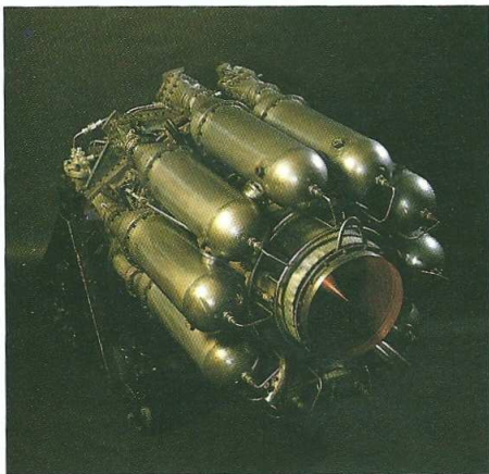
The Whittle W2/700 engine intended for the M.52
