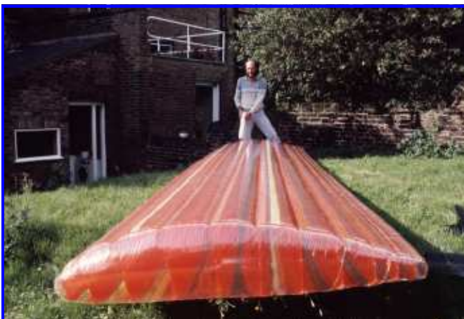
20' span prototype wing for Phoenix demonstrated by Ian
