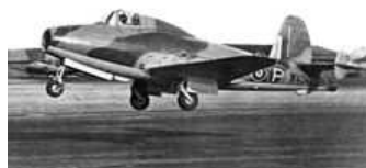
The Gloster E.28/39, the first British aircraft to fly with a turbojet engine
