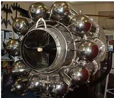
The W2/700 engine, or W.2B/23 as it was known to the Air Ministry. The W2/700 was the first British production jet engine, powering early models of the Gloster Meteor.
